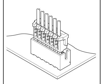
The twin U-slots (IDC slots), the 3-point insulation grip, and the distortion resistant disconnectable construction ensure a reliable connection even during severe environmental conditions.
