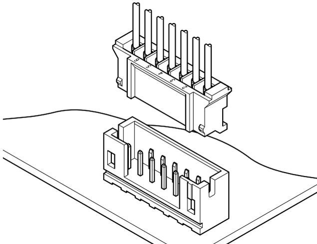
This is a thin, low-profile 2.0 mm pitch connector 8.0 mm in height after mounting and 4.5 mm in width. It is designed to meet the demand for high-density connection of internal wires to printed circuit boards. It is compact, highly reliable and low in cost.
