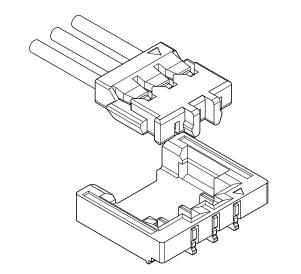
This ACHF connector is compact and low profile type, height 1.43 mm and width 4.95 mm, 1.2 mm pitch wire-to-board connector.
