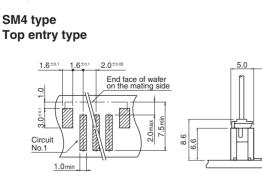
Note: 1. Tolerances are non-cumulative: ±0.05mm for all centers. 2. The dimensions above should serve as a guideline. Contact JST for details.
