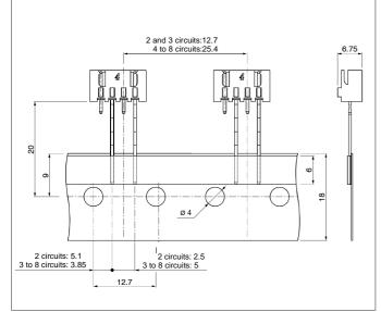
Note: Conforms to JIC C 0806 of "Tape packaging of components with unidirectional leads on continuous tapes".
