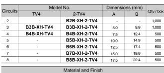
Post: Brass, copper-undercoated, tin-plated (reflow treatment) Wafer: TV4 type/ PA 66, UL94V-0, natural (white) 2-TV4 type/ Glass-filled PA 66, UL94V-0, natural (ivory)
