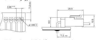
\*11.0 max. when used with the VR connector receptacle.
