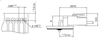
\*11.0 max. when used with the VR connector receptacle.
