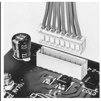
The ZH connector is very small with a mounting height of 5.6mm (.220") and a thickness of only 3.5mm (.138"). Contact retention lances on the housing make insertion easier, while the dimple at the center of the contact ensures reliable contact with the post.
