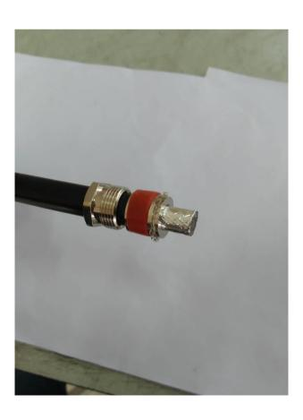
Use the blade to remove insulation, and keep a distance, the distance from 1 mm - 1.5mm
