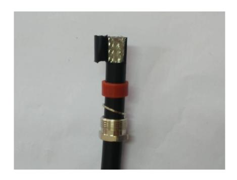
Step 2 Thick gasket set outside the shielding layer
