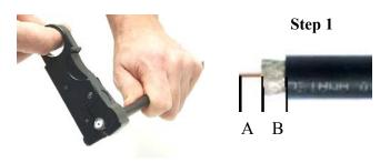
The cable after the stripping operation
