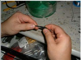
Push the strain relief to Rg174 cable
