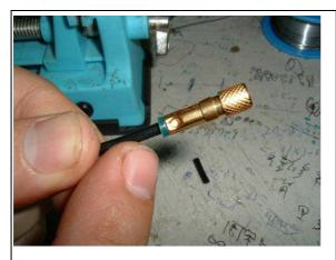
The crimping is special design to crimp this connector and BNC connector.
