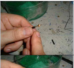
Cut the clear central cores plastic shielding. Cut approx. 3 mm off
