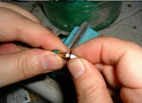
Push pin guide tube into the pin Press all parts tight together.
