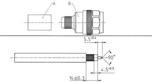
Preprare the cable according to the diagram and chamfer the center contact of the cable. If existant, cut the foil between the braid and the insulator of the cable together with the braid.
