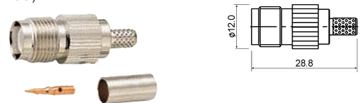
PLU010044 R/P TNC female crimp type gold-pin (RG58U/174U/178U)
