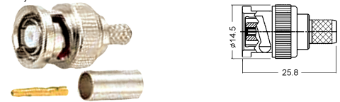
R/P BNC male crimp type gold-pin (RG58U/174U/178U)
